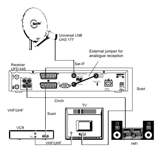
Connection of the DVB-S receiver to a TV set, a VCR and a HiFi system for receiving and recording digital satellite TV and radio channels.
